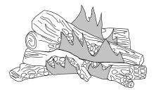
Figure 53 - Typical Flame Pattern for CDV37N/P(A,B) and CDV41N/P(A,B)
